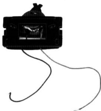
Alter Baßregler / Old roll-off filter
